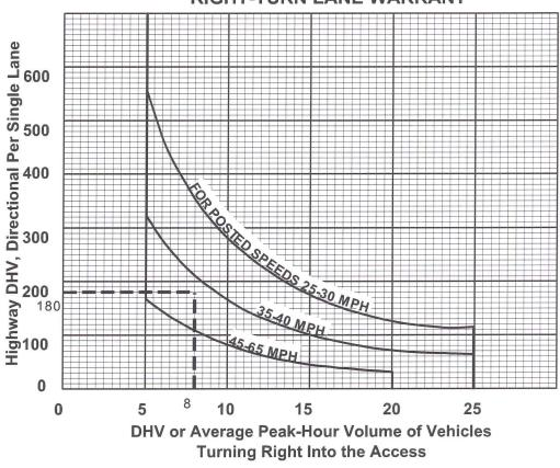
The single-lane DHV is  $0.5 \ge 360 = 180$  vph. Entering the right-turn warrant chart with 8 vph on the horizontal axis and 180 vph on the vertical axis gives a point of intersection below the 35-40 mph curve. A right-turn lane should not be considered at the intersection.
