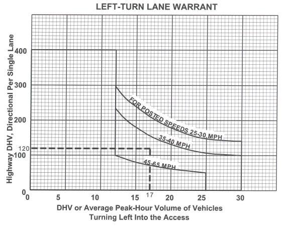
The highest single-lane DHV is  $0.6 \ge 200 = 120$  vph. Entering the left-turn warrant chart with 17 vph on the horizontal axis and 120 vph on the vertical axis gives a point of intersection above the 45-65 mph curve. A left-turn lane should be considered at this intersection after evaluation of all the above factors.
