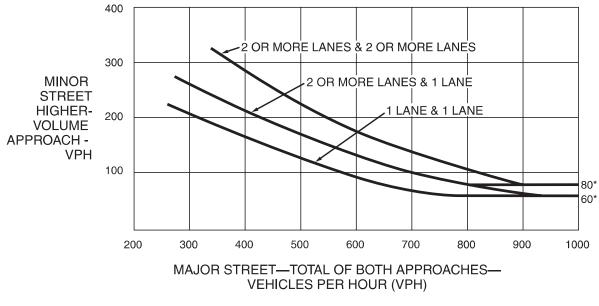
\*Note: 80 vph applies as the lower threshold volume for a minor-street approach with two or more lanes and 60 vph applies as the lower threshold volume for a minor-street approach with one lane.
