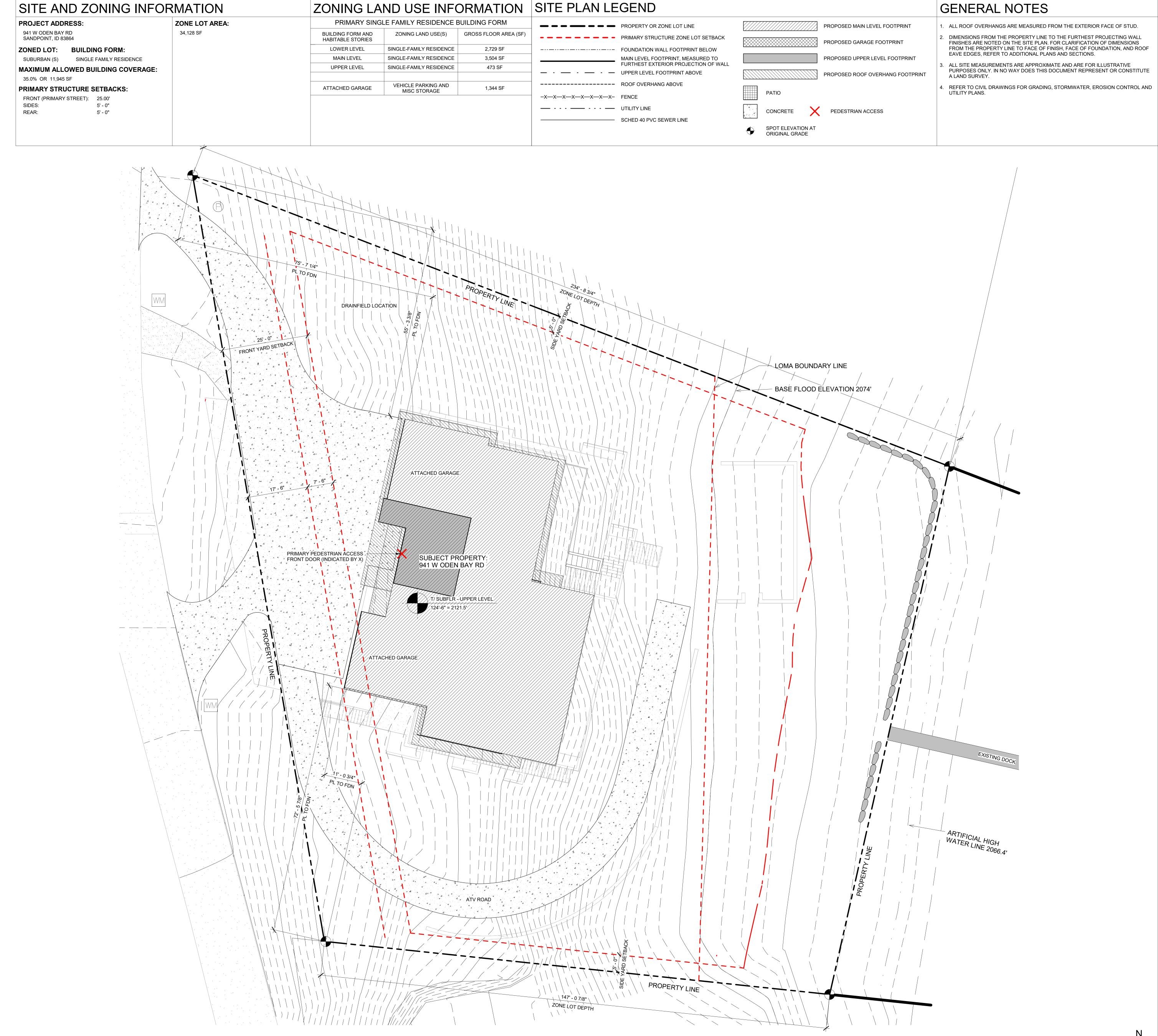
ALL ROOF OVERHANGS ARE MEASURED FROM THE EXTERIOR FACE OF STUD. DIMENSIONS FROM THE PROPERTY LINE TO THE FURTHEST PROJECTING WALL FINISHES ARE NOTED ON THE SITE PLAN. FOR CLARIFICATION OF DIMENSIONS FROM THE PROPERTY LINE TO FACE OF FINISH, FACE OF FOUNDATION, AND ROOF EAVE EDGES, REFER TO ADDITIONAL PLANS AND SECTIONS.
